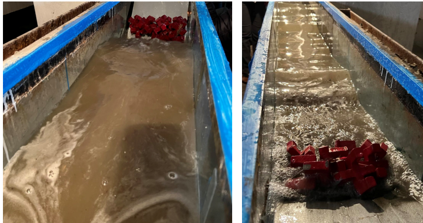
Fig. 7. Study of the wave dampening efficiency of fill on a slope with "Modified Hexablocks" and "Modified Tetrablocks" in a small hydraulic tray (10.0 m × 0.3 m × 0.70 m) (own research)
