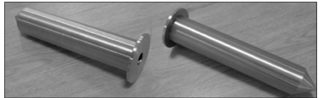
Rys. 6. Prototypowe emitory wykonane zgodnie z projektem Fig. 6. Prototype emitters made according to the design
