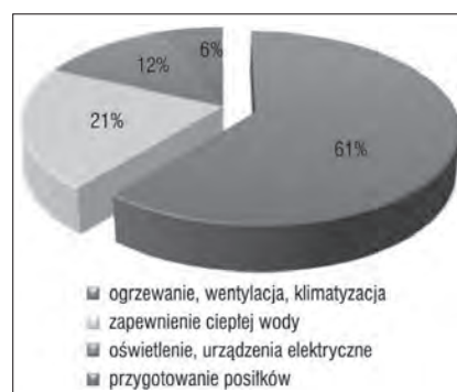
Rysunek 1. Struktura zużycia energii w hotelu [3] Figure 1. Diagram of energy consumption in a hotel [3]
