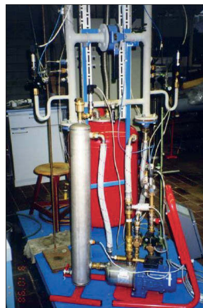
Rysunek 10. Stanowisko badawcze – system odgazowania próżniowego – Servitec prod. Reflex [36] Figure 10. Test stand – vacuum degassing system – Servitec manufactured by Reflex [36]
