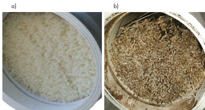
Fig. 4. PVDF membrane: a) unused polyvinylidene fluoride (PVDF) membrane; b) fouled membrane surface with visible contaminant deposits requiring chemical regeneration [24]
